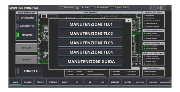
To carry out the automatic cycles a state machine (sequencer) is implemented. The sequencer determines the steps and conditions for transitioning from one step to another in the work cycle. To better understand the management of the software we can look at the HMI which in fact is divided into pages, each for each component and within them we will find consents, states and in some cases the commands.
