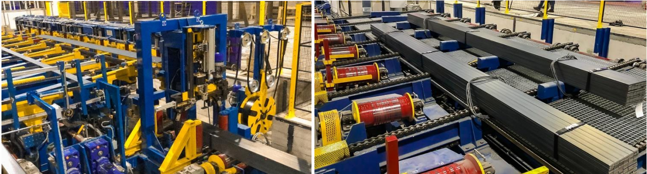
Figure 4&5 – Automatic strapping machine and bundles of strapped bars.
