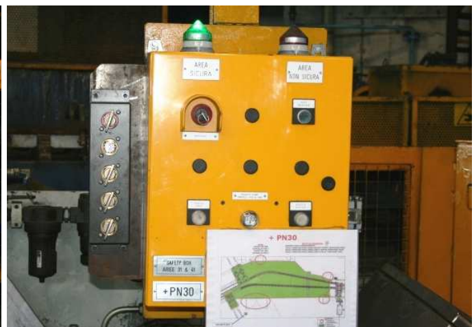
Fig. 13. Safety gates and removable fences controlled through released keys
