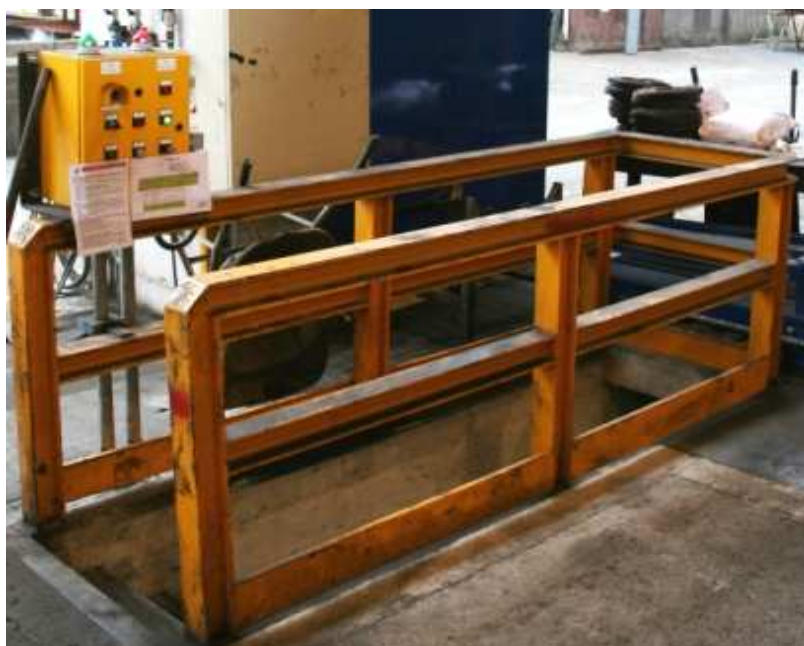
Fig. 15. Manhole controlled by safety system. Red light means running machine (unsafe area) – Green light means hole accessible. Green flashing light and buzzer means operator in hole.
