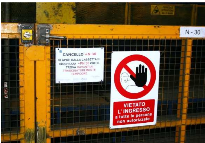
Fig. 13. Safety gates and removable fences controlled through released keys
