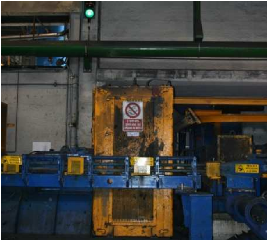
Fig. 16. Protection carter controlled through limit switch
