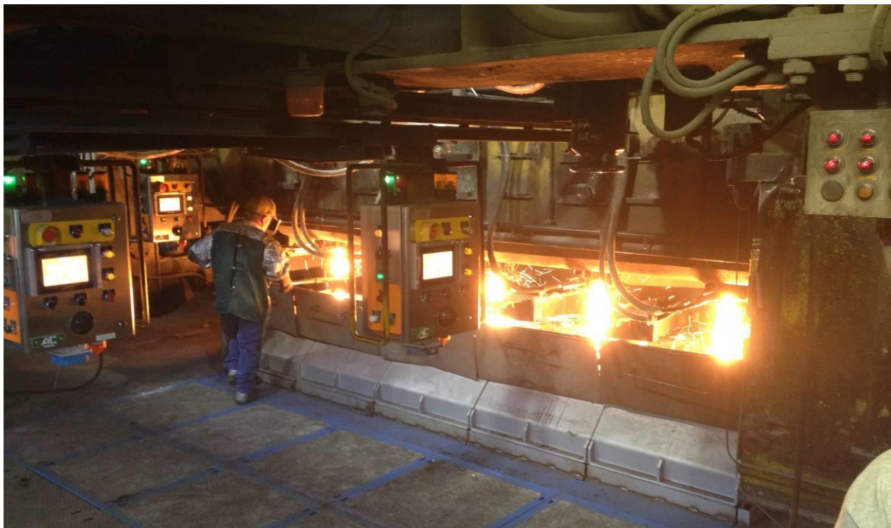
Overview of casting lines of CCM#1 (and related local control stations) during the start-up
