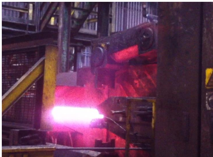
Dividing Shear at Cooling bed entry
